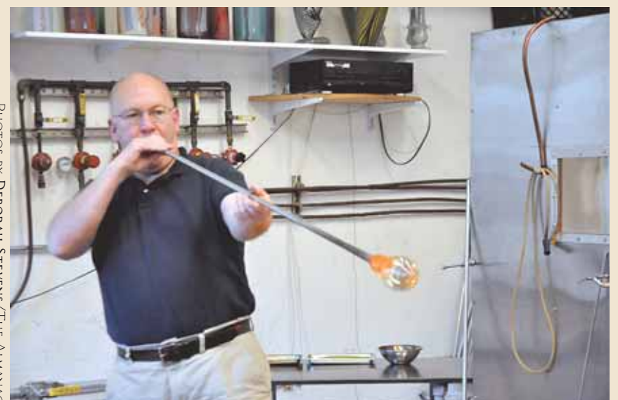
William Gudenrath starts to make the bottle by blowing the hot glass.
