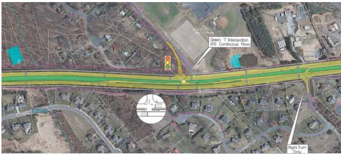
A redesign of the Route 7-Utterback Store Road intersection that will happen with the widening of Route 7. The design will make the eastbound lanes part of a continuous intersection, not governed by a traffic signal.
