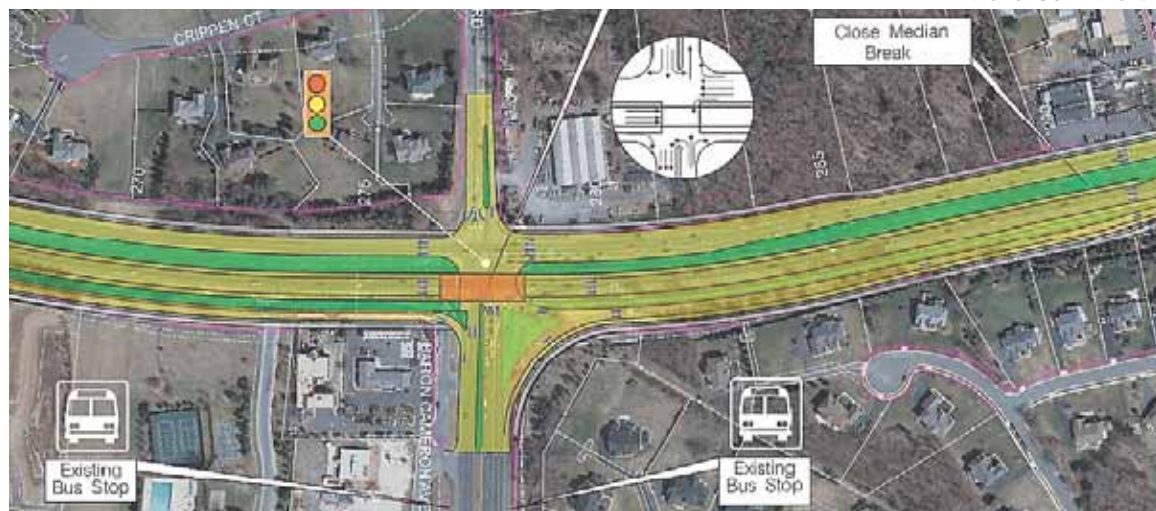
The intersection of Route 7 and Baron Cameron Avenue will have an eastbound flyover addition with the upcoming widening of Route 7.
