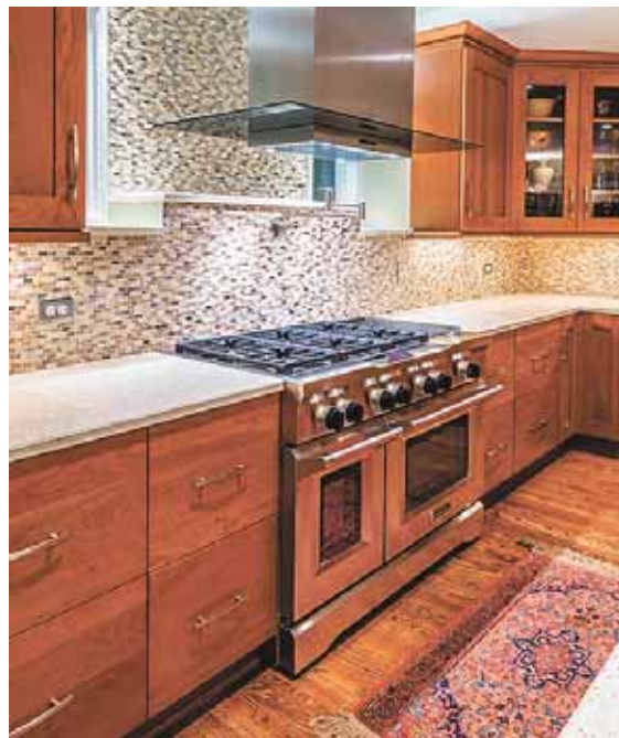
A south-facing bump-out accommodates a cook-top ventilator flanked by transom windows. The concentrated small space solution enlarges the cook’s work triangle and creates an additional source of natural light.
