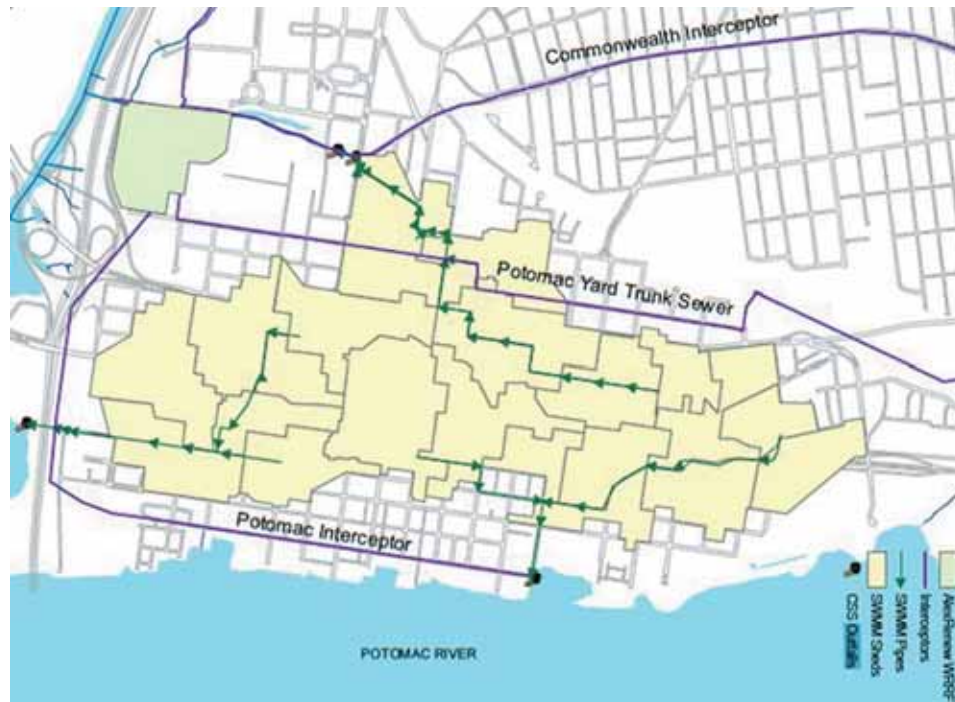
Old Town has a total of four outfalls, three of which dump raw sewage into Hunting Creek. One is on Royal Street and two are on Duke Street.
