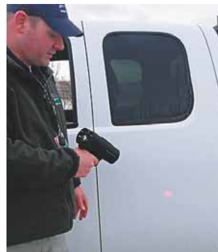
The laser gun shoots a small red dot that is very effective and safe at scaring off birds.
