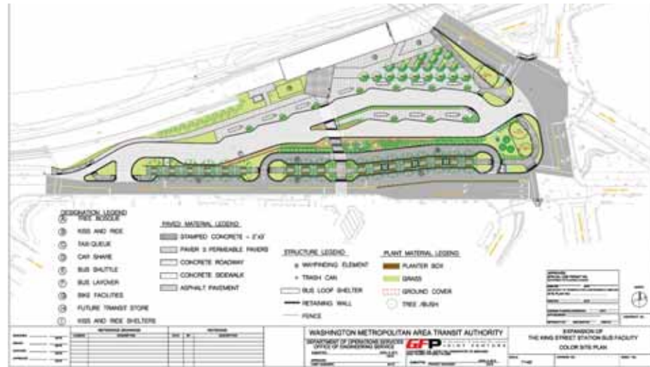
The new site plan for the King Street Station features a one-way Kiss & Ride loop and an "island" for three more bus shelters.
