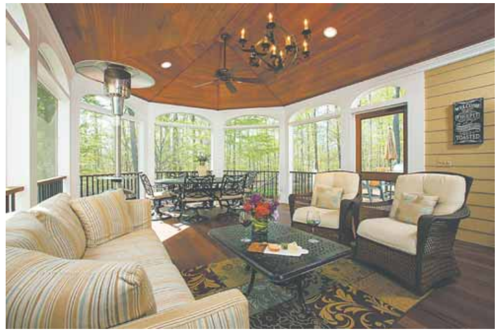
The spacious new screened porch demonstrates how highly durable materials can be shaped to meet demanding aesthetics. The Ipe decking chosen for the porch flooring is one of the most enduring natural hardwoods offered for outdoor surfaces; installed in a tongue-and-groove pattern, it keeps out bugs more effectively than screen mesh. The fiberglass charcoal screen, likewise, makes it hard to see the porch interior from the outside.
