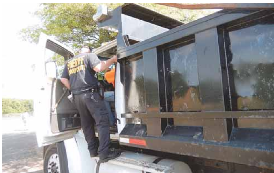
Loudoun Sheriff's Deputy Bart Foster inspects this dump truck and trailer. The truck's two brakes in front and one in the rear were out of adjustment, so it was sidelined for repairs.
