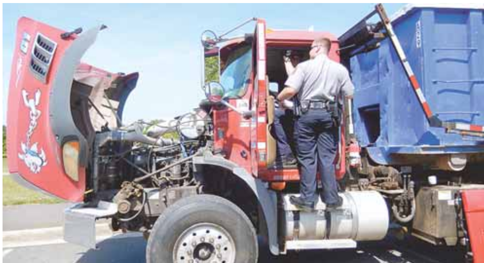
Motor Carrier Safety Officer Shawn Regan (in cab) and PFC B.P. Woehrle (outside the cab) inspect a roll-off truck hauling construction debris. They checked its gauges, low-air warning devices and signals and discovered some of its brakes were out of adjustment.
