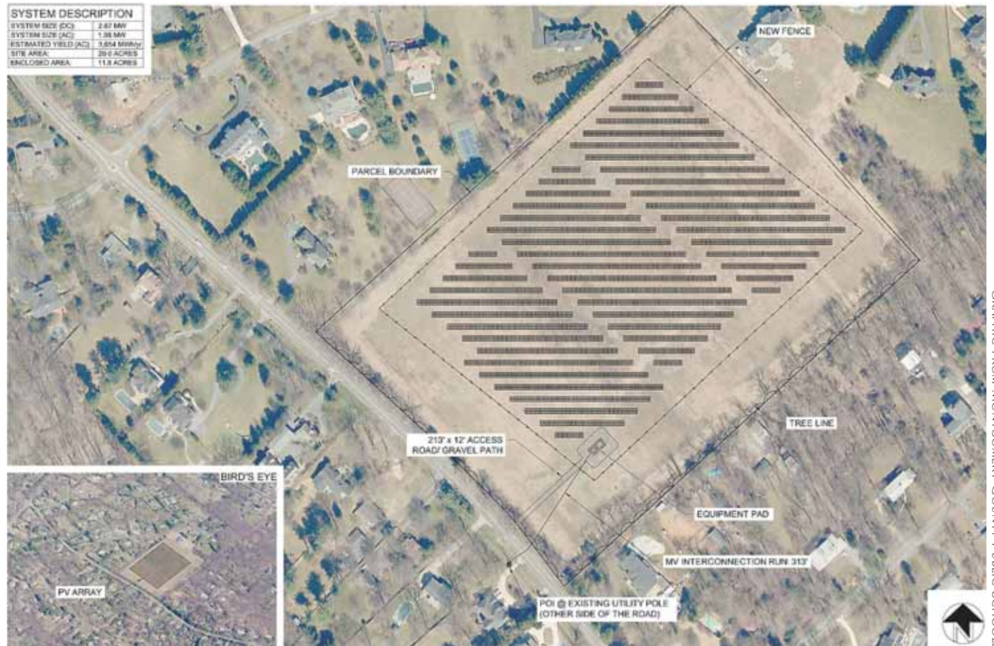
Solar array as envisioned for the Brickyard Road site; ground mounted panels would cover 12 acres of the site, with a chain link fence topped by barbed wire surrounding.
