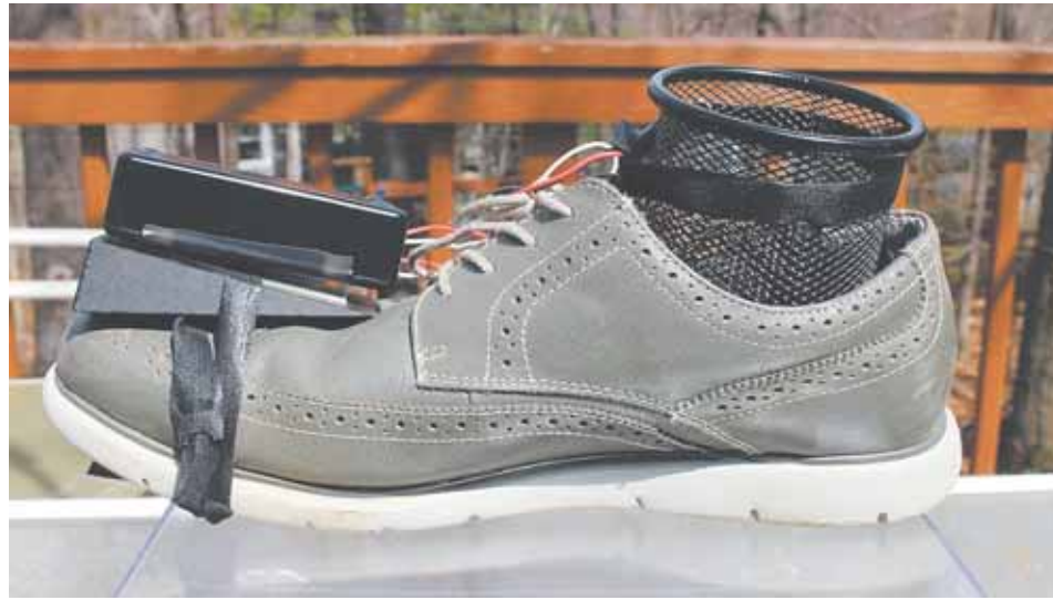
"Stride," a design by South Lakes High School sophomore Srijay Kasturi, senses objects up to six feet in front of the wearer and transmits a vibration to their ankle to warn them.
