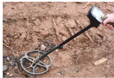
Kabat's metal-detector can accurately spot a target down to the size of a small coin.
