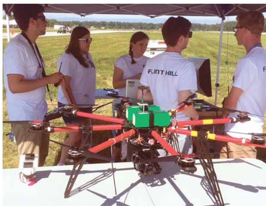
Flint Hill School students designed, built and programmed an air vehicle capable of autonomous flight over a distance of more than three miles.
