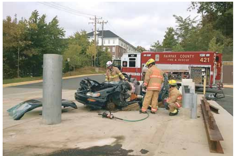
Vehicle extrication crew just removed the roof of a wrecked car. They show how they would use a hydraulic spreader to lift the dashboard and steering column off a trapped driver.
