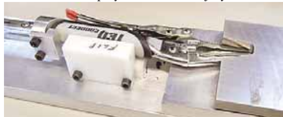
Special tooling turns raw materials into market Auto-Grip pliers.
