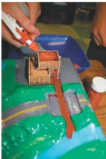
The red dye is effective in showing the downstream flow.
