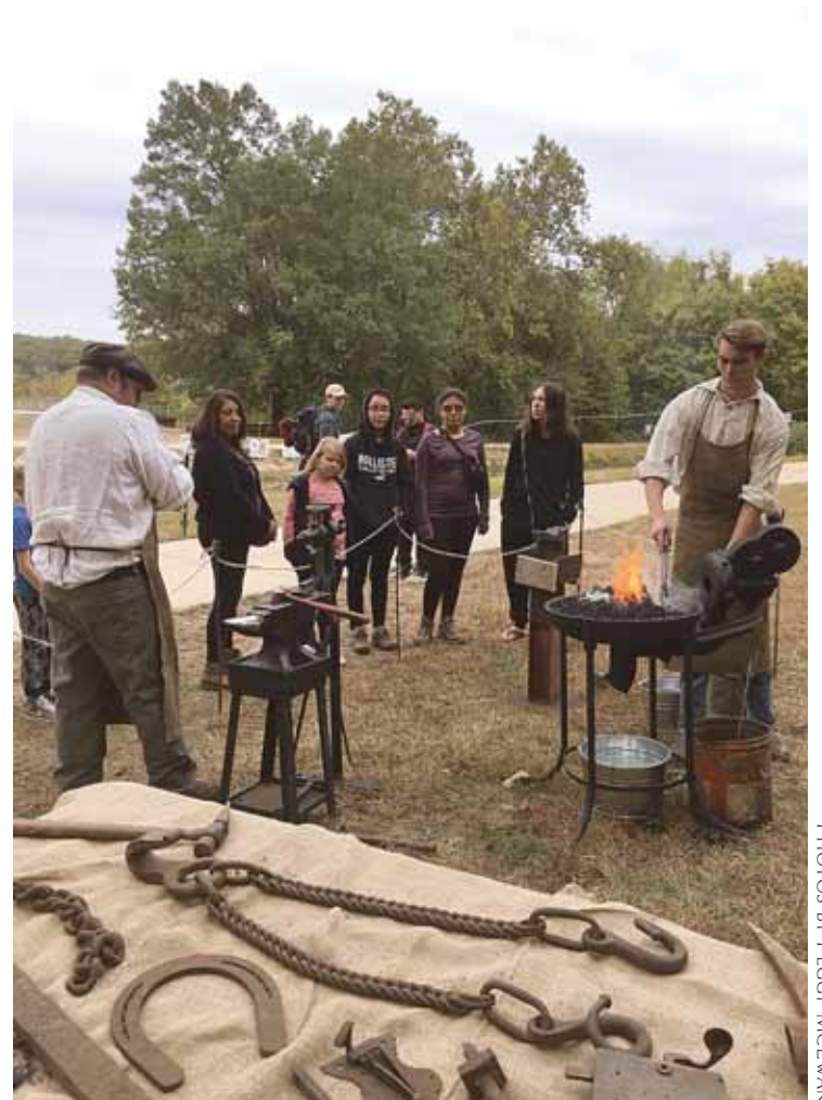
Apprentice blacksmith Josiah Bloom runs bellows to supply oxygen to the fire while blacksmith Eric Johnson explains his craft to onlookers at Great Falls Park.
