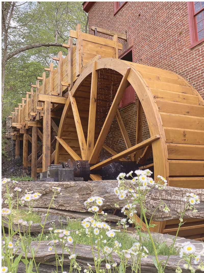
Water will flow into the elevated flume and over the wheel of the mill.
