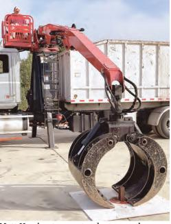
Matt Harris, stormwater dept. uses the knuckleboom to pluck a brick and move it to the target circle on the opposite side of the truck.
