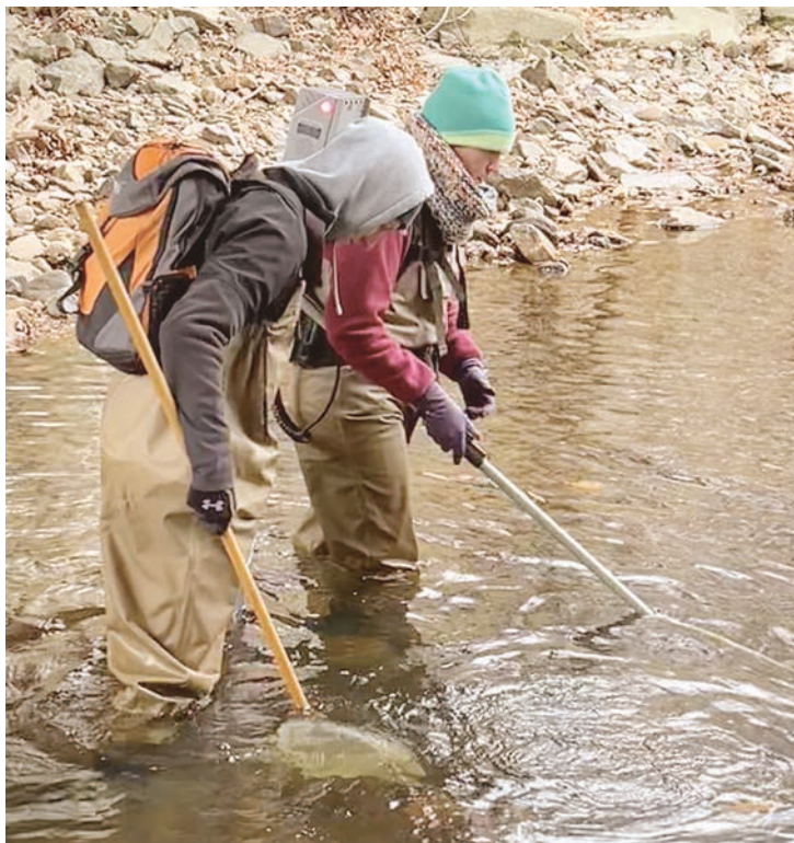
Tim Jones and Courney Hauler work together to stun and survey fish and eels, using an electro-fisher unit.
