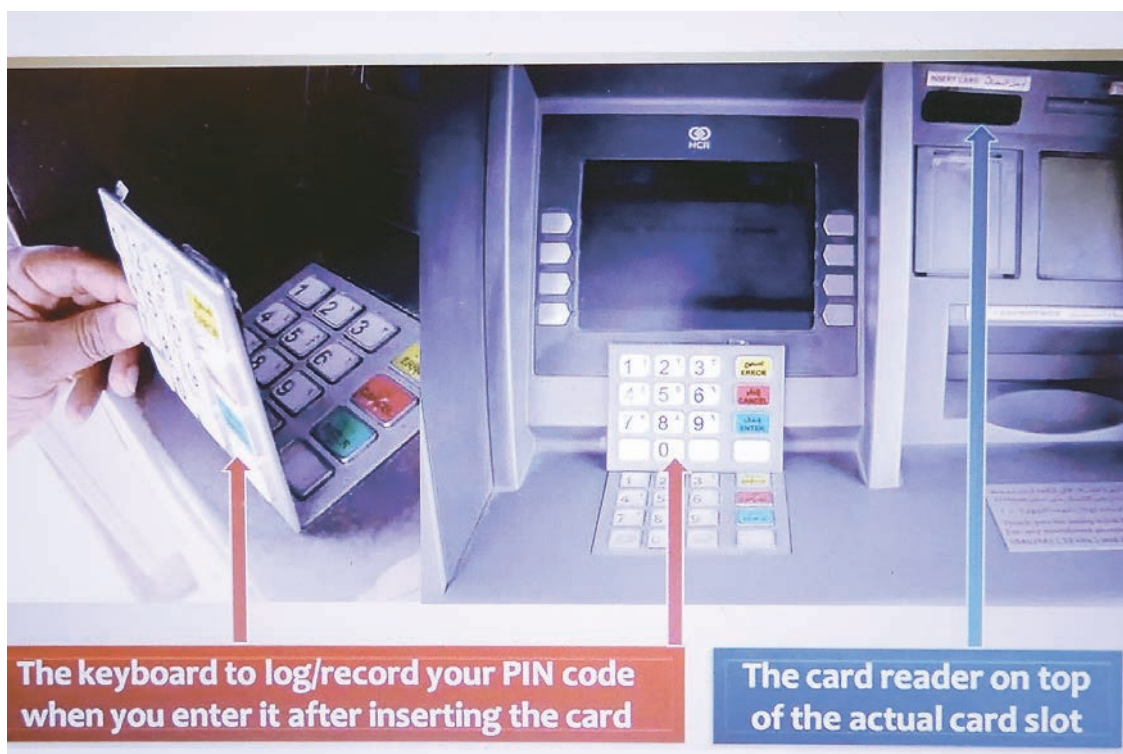
An example of the inside of a credit-card skimmer at a bank ATM.
