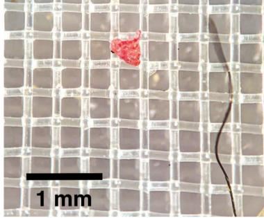
Magnified image of microplastics (a fragment and a fiber) collected at Four Mile Run, seen against the filter mesh screen.
