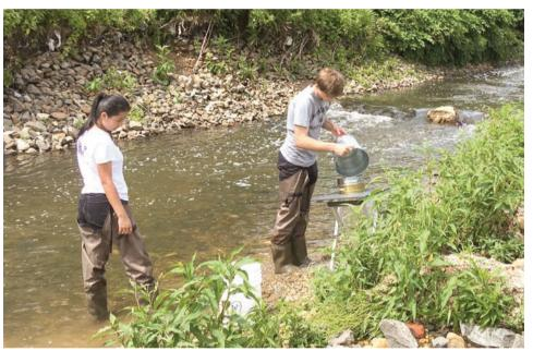
Researchers at Four Mile Run pour a water sample through a sieve to collect microplastics for lab analysis.
