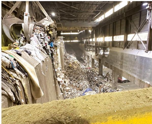
Starting on the "tipping floor," trash trucks (lower right) bring garbage from collection routes or the I-66 transfer station to the Covanta plant where the amount of trash and dust would drive any determined housekeeper insane.
