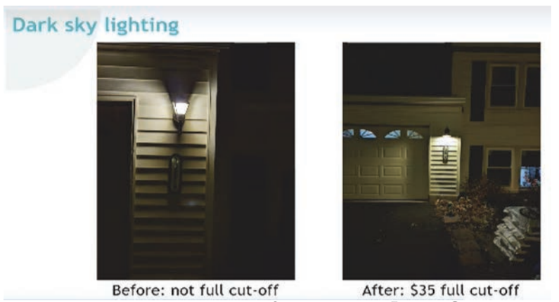
Protect the night sky: Residents can use fixtures with full cut-out, meaning light is not emitted above the bottom of the fixture.
