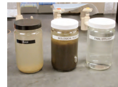
Jars of water at Alexandria’s wastewater treatment plant showing water that came in and treated water that went out.
